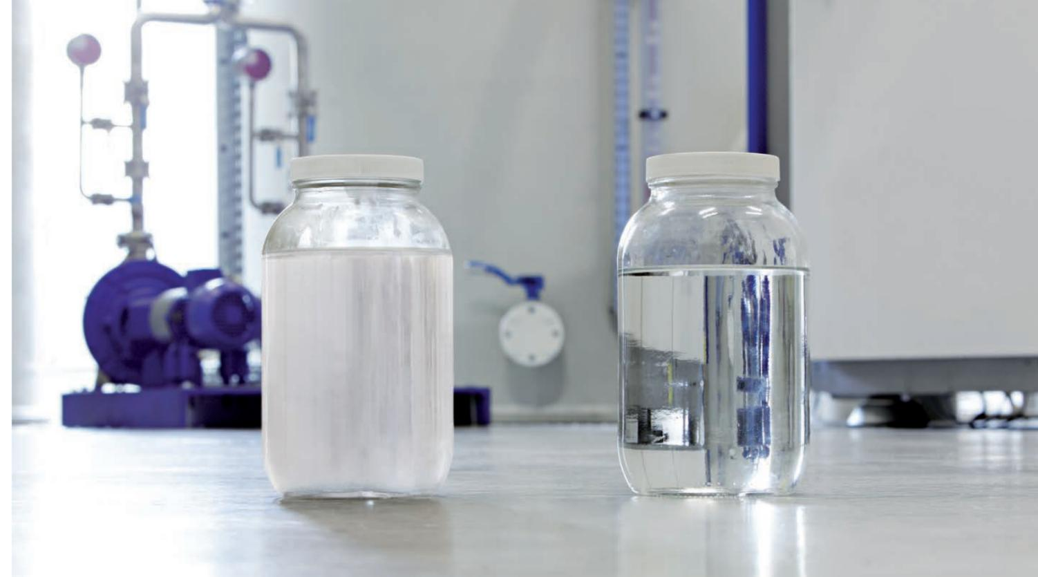
A simple optical comparison of distillate from conventional vacuum evaporators and VACUDEST Clearcat shows that the future proof Clearcat condensations system is setting benchmarks regarding quality of the treated industrial wastewater. The result is crystal clear and almost free of oil.
