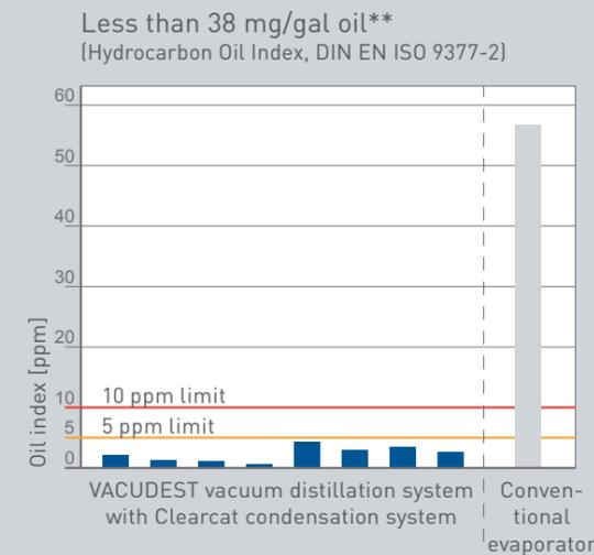
The future proof Clearcat condensation system allows better reduction of the oil index than conventional evaporators combined with post treatment steps. This allows the oil content to be reduced to less than 38 mg/gal.
