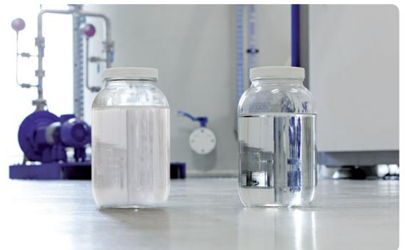
A simple optical comparison of distillate from conventional vacuum evaporators and VACUDEST Clearcat shows that the future proof Clearcat condensations system is setting benchmarks regarding quality of the treated industrial wastewater.
